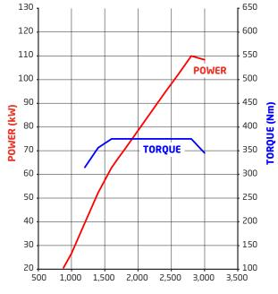
**ENGINE SPEED (RPM)**
