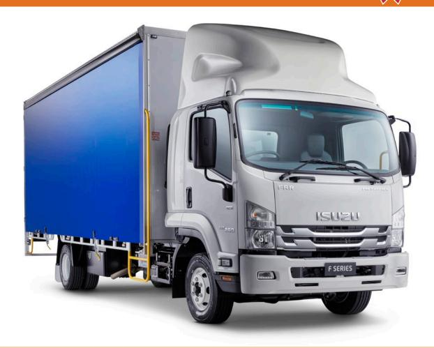
10 pallet (nominal) curtainside body / Easy glide curtains with quick release "Lightning" latches / Lightweight side gates / 3mm checkerplate floor and headboard with load restraints / Safety yellow coloured body steps and grab handles / Removable rear step facilitates tailgate loader installation / Underbody mounted storage box / LED lighting for body interior and access steps / Genuine Isuzu roof mounted air deflector / Digital reversing and body interior camera / Daytime running lamps
