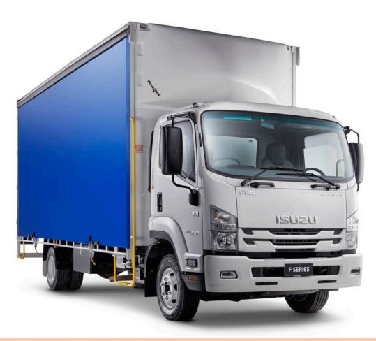
10 pallet (nominal) curtainside body / Easy glide curtains with quick release "Lightning" latches / Lightweight side gates / 3mm checkerplate floor and headboard with load restraints / Safety yellow coloured body steps and grab handles / Underbody mounted storage box / LED lighting for body interior and access steps / Body mounted air deflector / Digital reversing and body interior camera / Daytime running lamps
