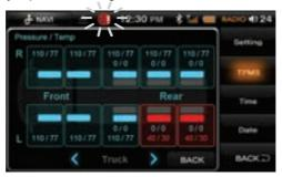
B. Flashing icon, warning buzzer(1Sec intervals) and warning screen. Tyre pressure is 30% lower than minimum level set. Re-inflate tyre to correct tyre pressure as soon as possible.
