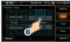
B. Select the location of installed TPMS sensor.
