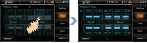
Drive the vehicle until all sensor readings are displayed.
