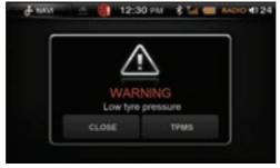
Press TPMS button to check which tyres are low on pressure. The location of the under inflated tyre will glow Red. Press Close to turn off warning buzzer.
