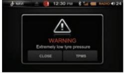
Press TPMS button to check which tyres are low on pressure. The location of the under inflated tyre will glow Red. Press Close to turn off warning buzzer.
